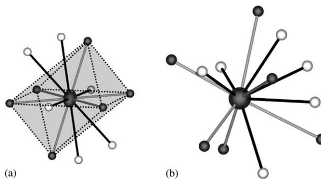
Fig. 5. Ba(1) is connected to six N(1) (gray) and N(2) (black) with distances 3.320(6) and 3.011(6) Å. The coordination of Ba(1) with N(2) is a significant distorted octahedron. Ba(2) is also connected to six N(1) and six N(2) with distances between 2.811(6) and 3.449(6) Å. Therefore both Ba atoms have a 6 + 6 coordination sphere. (a) Coordination sphere of Ba(1) and (b) coordination sphere of Ba(2).
