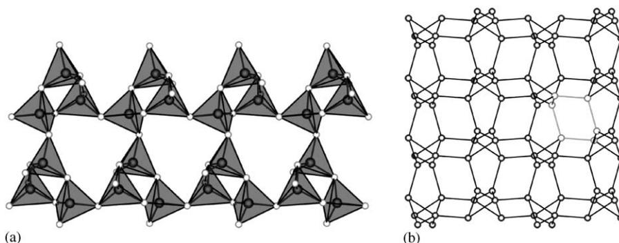
Fig. 6. The left figure is a section of the  $\text{BaP}_2\text{N}_4$  structure. It shows characteristic 3-rings connected by corner sharing tetrahedra forming 7-rings (view along [001], Ba atoms are left out). The right figure shows the 6-rings (view along [010]). For reasons of clarity only the P-atoms are shown. One 6-ring is marked light gray. (a) 3-rings and 7-rings and (b) 6-rings.
