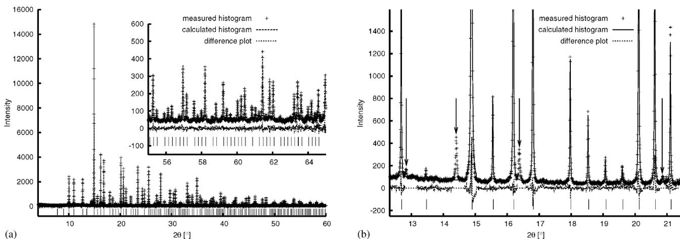
Fig. 2. The synchrotron measurement resolves the diffraction pattern of  $\text{BaP}_2\text{N}_4$  and the unknown minor phase completely. The inset shows the good signal-to-noise ratio at high angles. (a) Whole diffraction pattern of  $\text{BaP}_2\text{N}_4$  and (b) Histogram of  $\text{BaP}_2\text{N}_4$  and minor phase (marked with an arrow).
